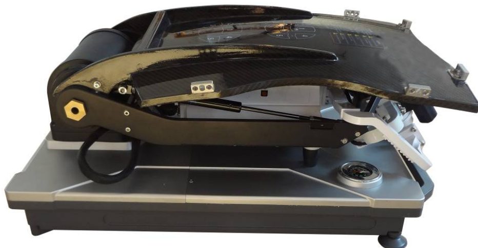
Figure 2. The stowing status of 1.0m flyaway antenna
