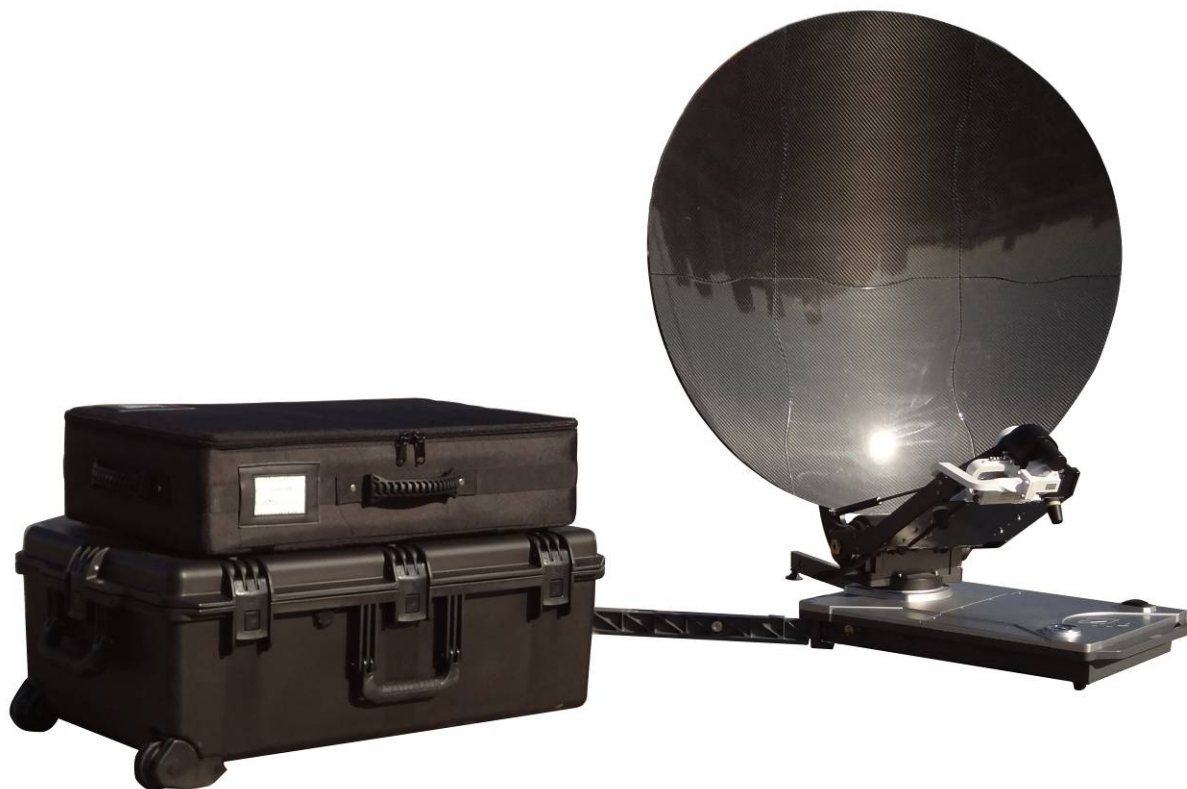
Figure 1. The working status of 1.0m flyaway antenna
